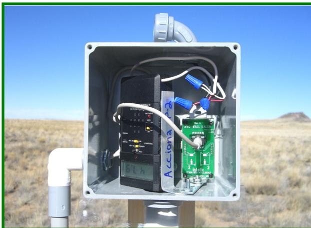
Figure 2. Balun system in use (the device on top of the enclosure is a homemade light sensor).
